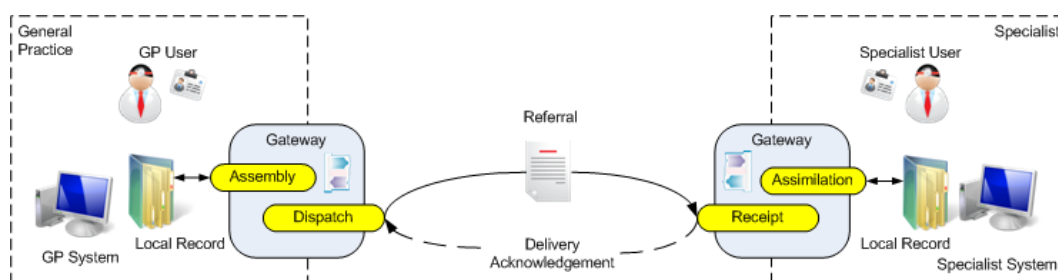
Figure 4 High Level Solution View (Interim Solution State)
